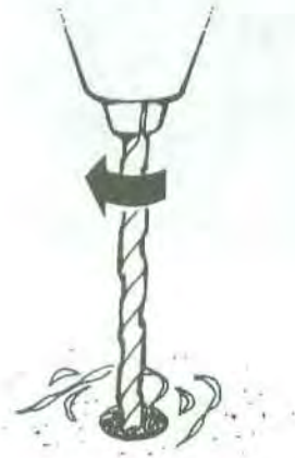
2. Drill hole in stud
